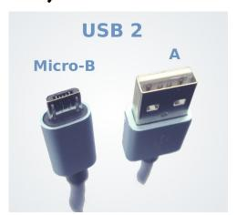
The USB cable you're most used to seeing is probably the USB Type-A to Micro-B cable. This is used by most Android smartphones to charge and transfer data. The connectors use only 4 wires, two for data and two for 5V power. These are limited to the USB 2.0 speed of 480Mbit/s
