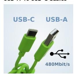
There are two varieties of USB-A to USB-C cables that allow you to plug your USB-C phone into a computer with USB-A ports. If you look closely at the "A" connector you can tell the difference. If it's blue and/or has the 5 extra contacts, it's capable of USB 3 speeds of 5 or 10Gbit/s; otherwise it will limit you to the USB 2 speed of 480Mbit/s. The SuperSpeed cables might have the SS trident or SS 10 trident logo on them like tha amazon cable on the bottom left.
