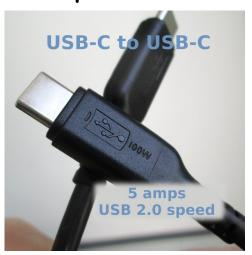
"USB PD" is the new protocol that allows devices to negotiate higher voltages and current for charging. All USB-C to USB-C cables support the PD protocol, but most limit you to 3A = 60W charging (depending on the devices on each end). But if you want to charge at over 60W there's another option that could apply to any of the above cables. There's no logo, but the cable literature should state that it supports "100W," or "5A" or "5 amps."
