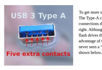
To get more speed, USB 3.0 added 5 more wires to the connectors. The Type-A connector looks the same, but there are 5 more connections deep inside. It might sport the SS trident logo on the right. Although you've probably used USB 3 flash drives that fit this connector and take advantage of the extra speed, you may have never seen a "SuperSpeed" cable with the end
