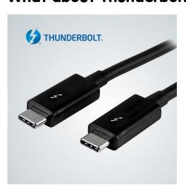
Thunderbolt 3 cables use the same connectors as USB-C. The specs on the wiring for Thunderbolt are tighter than for USB-C cables. Generally, you can successfully use Thunderbolt cables for a USB-C power and SuperSpeed data connection, but longer "active" thunderbolt cables (over .5 meters) will be slow, falling back to only 480Mbps. Like standard USB-C cables they can charge at 3A/60W, some up to 5A/100W.
