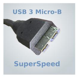
This cable with this Type Micro B connector on one end and a Type A on the other is a "SuperSpeed" cable capable of 5Gbit/s and 10Gbit/s, depending on the age of your devices. Cables under 1 meter long that bear the older SS trident logo are just as good as newer cables with the SS 10 logo. The protocol changed to get the extra speed, but the cables are the same. These cables are seldom used
