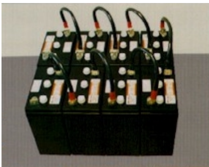
Battery bank composed of 6-volt batteries wired to produce 48 volts. (Do not try this at home.)
