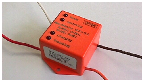
Charge controller— M-8 is part of JAARS starter system
