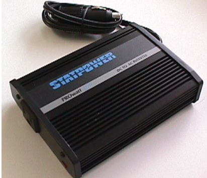
Inverter—Statpower ProWatt 250 is part of JAARS starter system
