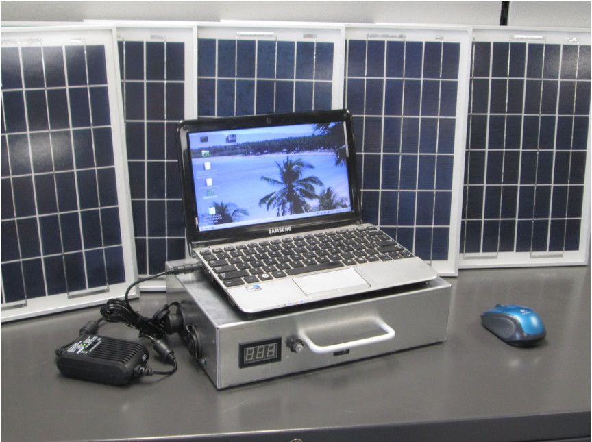
Villager III powering a convertible tablet with a DC-DC adapter
